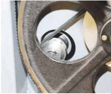
You swap the belt to alter to either of the two speed ratios
